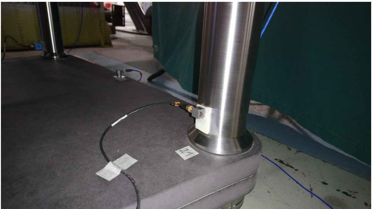
Figure 6. Golia rack during modal tests – Point 21.
